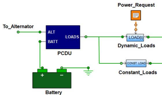
Figure 6. EcosimPro PCDU, battery and loads model
