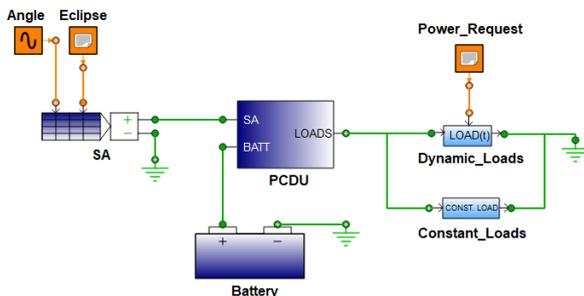
Figure 7. EcosimPro generic SEP system schematic
