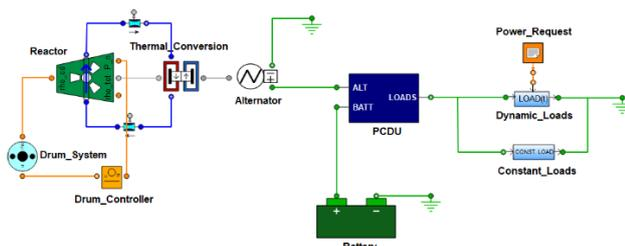
Figure 2. EcosimPro schematic of a Rankine NEP system
