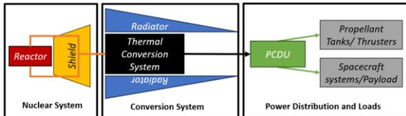
Figure 1. Schematic of a generic NEP system
