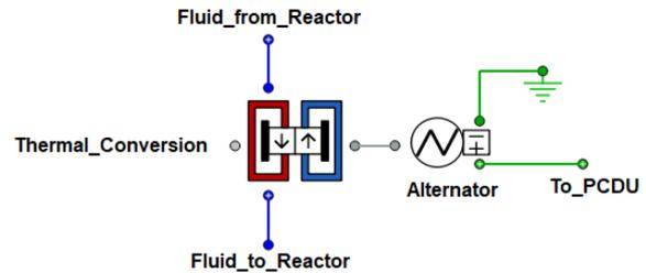
Figure 5. EcosimPro thermal conversion system model
