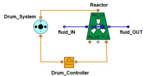
Figure 3. EcosimPro full nuclear reactor system model
