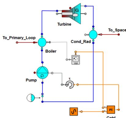
Figure 4. EcosimPro secondary fluid loop model
